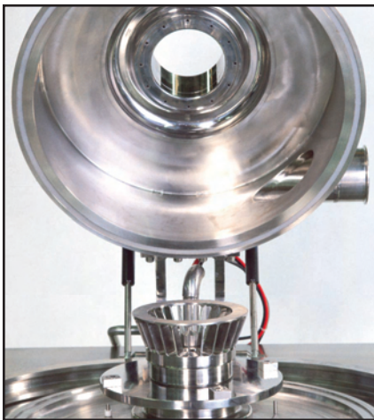
Internal view of Mikro-ACM® air classifying mill CIP design.
