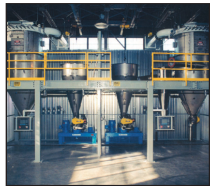
Our Toll Processing Facility features Mikro-ACM® air classifying mill systems for fine grinding.
