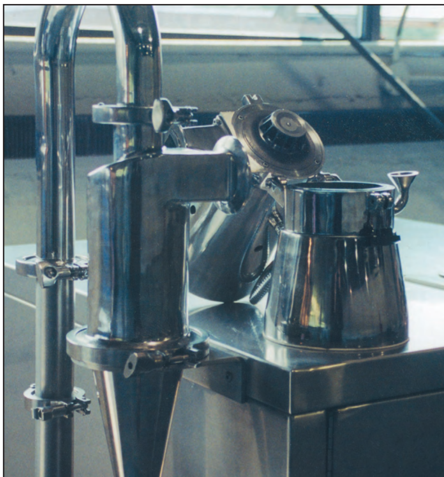
Mikro-ACM® air classifying mill model 1.
